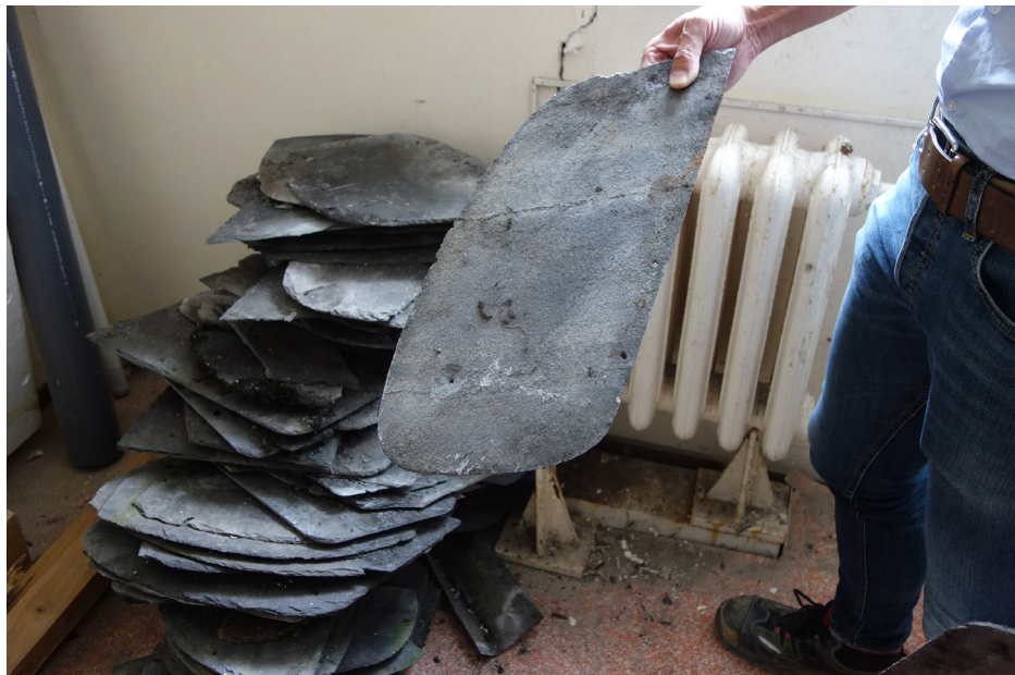
Survey of potentially reusable materials : slate tiles- Wiltz © Rotor
